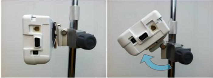
For a setup where it is desired to instead tilt the Monitor downward, remove the screws shown below, rotate the clamp 180°, and screw the clamp back down onto the plunger plate.
